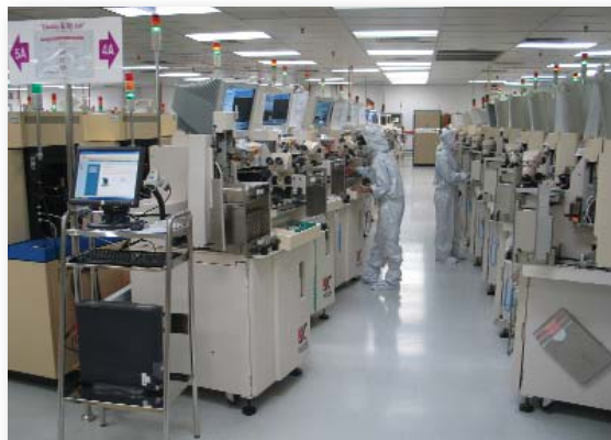
The wire bonding line at STATS' ChipPAC's Malaysian facility
